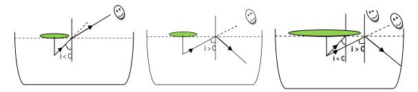
• We can find the critical angle of the medium (Water) by this experiment. To calculate critical angle, we have to use trigonometric ratios in the right angled triangle.
