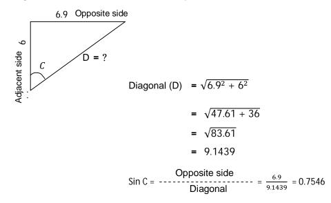
→ Sin C = Sin 48.99° It means the critical angle value is  $48.99^{\circ}$  (approximately  $49^{\circ}$ )
