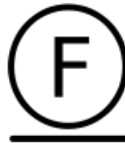
Gentle cleaning with hydrocarbon solvents
