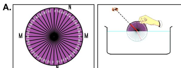
Take a circular metal disc. Cover with white chart. Mark one line as NN which is normal to the another line marked as MM. Here MM represents the line drawn along the interface of two media and NN represents the normal drawn to this line at 'O'. Take a protractor and place it along NN (its centre coincides with O). Then mark the angles from  $0^\circ$  to  $90^\circ$  on both sides of the line NN. Repeat the same on the other side of the line NN.
