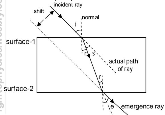
The angle between the actual path of ray and refracted ray is called angle of deviation ( $s$ ).
