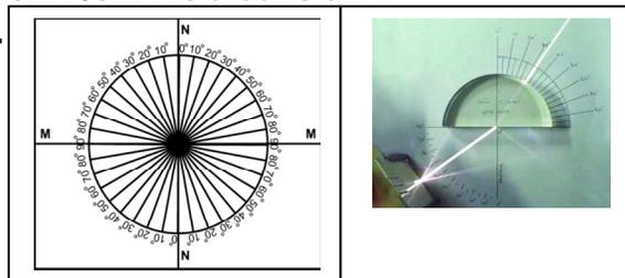
**Procedure:** Take a wooden plank. Cover with white chart. Draw two perpendicular lines, passing through the middle of the paper. Mark one line as NN which is normal to the another line marked as MM. Here MM represents the line drawn along the interface of two media and NN represents the normal drawn to this line at 'O'.
