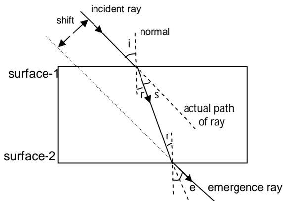
The perpendicular distance between the incident ray and emergence ray is called as lateral shift, if the slab is placed horizontally on the plane.
