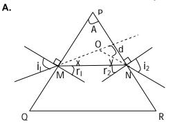
Place a white paper on a drawing board and arrange clips at is four ends. Place a prism on the paper so that the triangular shape touches the paper. Draw the boundary line with pencil. Name the vertices as P, Q and R. Measure the angle of the prism at 'P' and note down it as 'A'.
