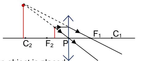
When object is placed between F<sub>2</sub> of P of a concave lens, the image is formed at the object side between focus and optical center. The image is virtual, erect and diminished.
