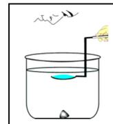
Keep a black stone inside the vessel at its bottom. Now pour water into the vessel up to a height (equal to 'f'). Now dip the lens horizontally using a circular lens holder. Set the distance between stone and lens that is equal to or less than focal length of lens. Now look at the stone through the lens. We can't see the image of stone.
