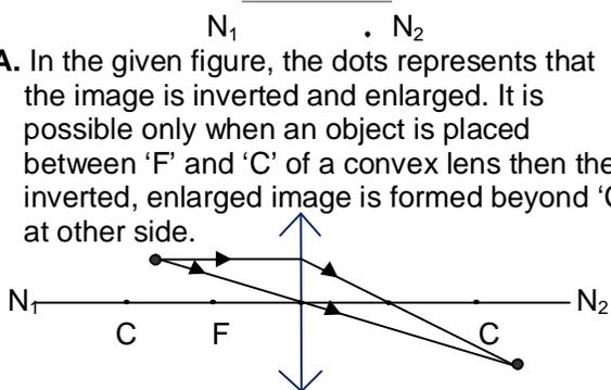
A. In the given figure, the dots represents that the image is inverted and enlarged. It is possible only when an object is placed between 'F' and 'C' of a convex lens then the inverted, enlarged image is formed beyond 'C' at other side.
