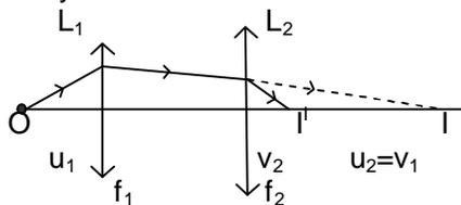
Let an object 'O' is placed at a distance  $u_1$  from the lens  $L_1$ . Assume that the image 'I' can be collected at a distance  $v_1$ .
