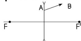
A. The incident ray which is parallel to the axis of a concave lens, seems to be diverges from the focus after refraction.
