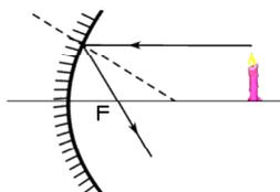
(ii) A ray that passes through the focal point of the mirror will travel parallel to the axis after reflection.
