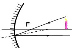
(iii) a ray coming from the tip of the object going through the centre of curvature to meet the mirror, it will get reflected along the same line.
