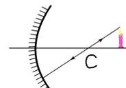
(iv) Along with these three Rays 'the ray which comes from the object and reaches the pole of the mirror' is also useful in drawing ray diagrams. For this ray, the principal axis is the normal.
